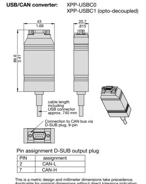
This is a metric design and millimeter dimensions take precedence. Applicable for nominal dimensions without direct tolerance indication: DIN ISO 286  $\pm$  IT 13. Refer to product datasheet for installation and safety instructions.
