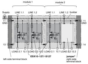
12.1, 12.2 status indication SF  $\overline{\text{OV}}$ =OK 13, 14 reset input RE ( group reset), +24V falling edge \*Caution: unused slots have to be fitted with jumpers
