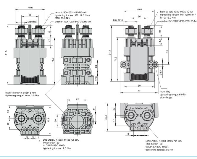
Mounting method 1 including side flange (50 mm hole spacing) and M4 screw terminals
